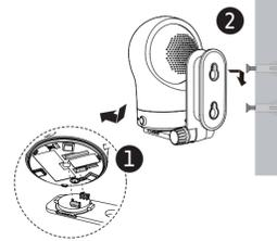
5. You can maximize your baby unit's viewing angles by tilting the wall mount bracket. Hold the baby unit, and then rotate the knob in anticlockwise direction. This will loosen the joint of the wall mount bracket. Tilt your baby unit up or down to adjust to your preferred angle. Then, rotate the knob in clockwise direction to tighten the joint and secure the angle.
