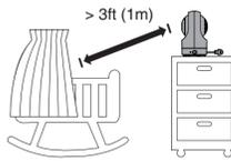
2. Adjust the angle of the baby unit to aim at your baby. Refer to the online help topics on how to use the Pan/tilt and Zoom functions of the baby unit.
